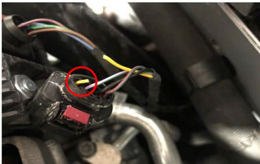
Figure 1. Wire is broken at G31 sensor.
