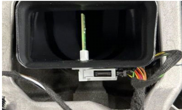
Figure 1. Harness routing prone to damage in assembly.
