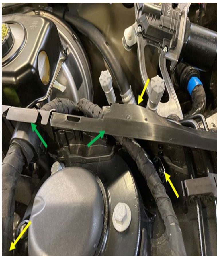
Figure 1: Plenum chamber covers (green arrows).
