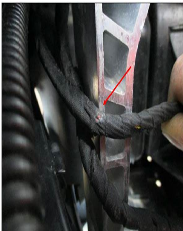
Figure 1. Example of parking aid harness that has chafing.
