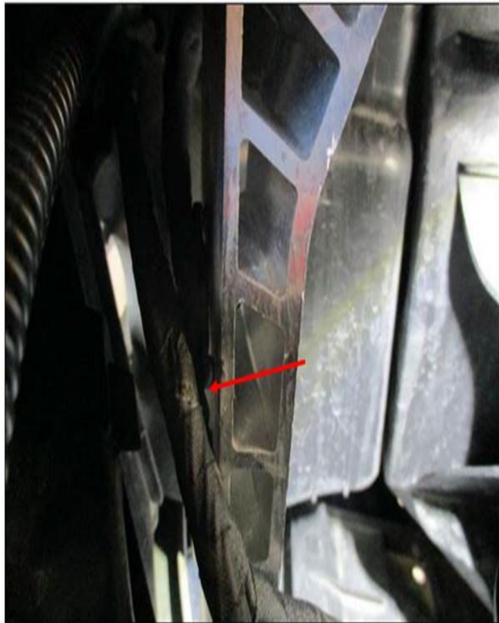
Figure 2. Example of parking aid harness that has chaffing.
