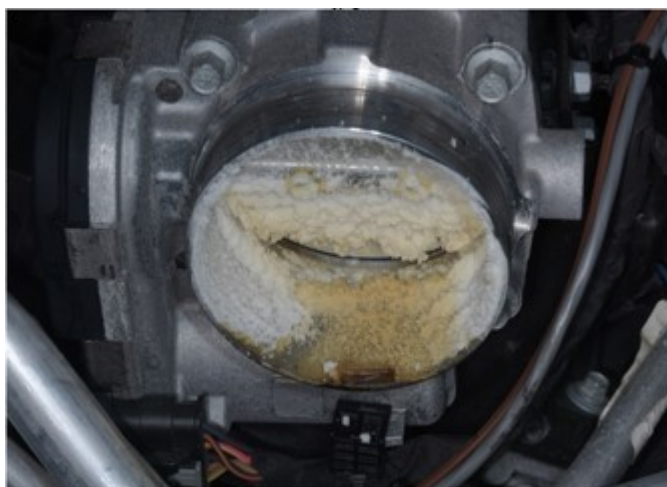
Fig. 1 Iced Throttle Body
