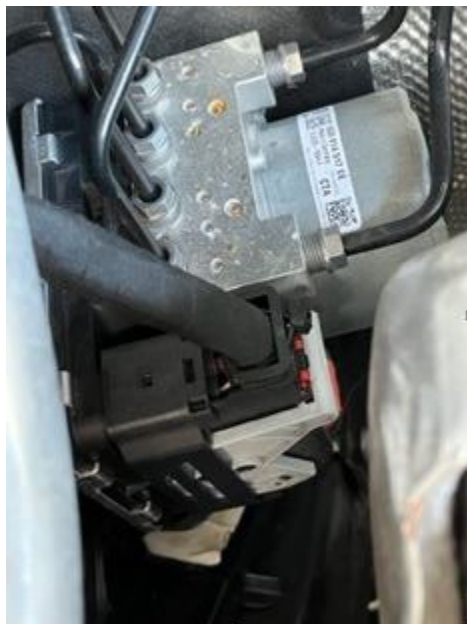
Figure 1: ABS hydraulic unit / ABS control unit connector.
