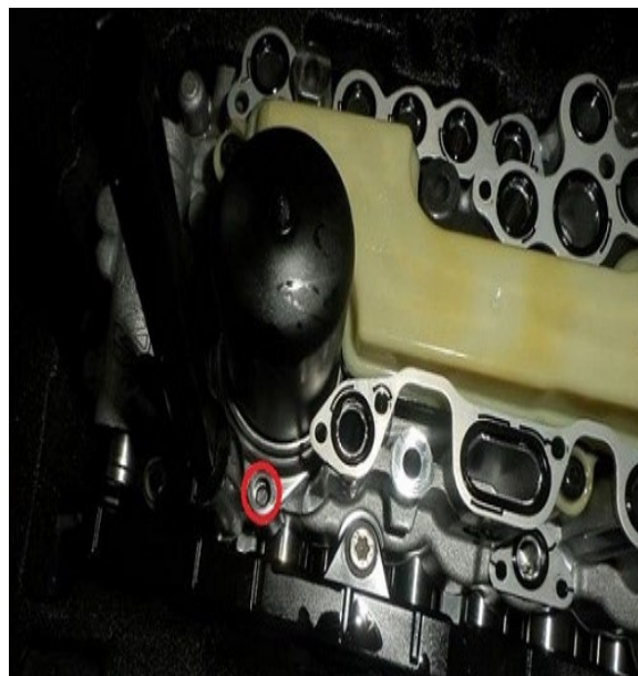
Figure 5. The bolt head is missing.
