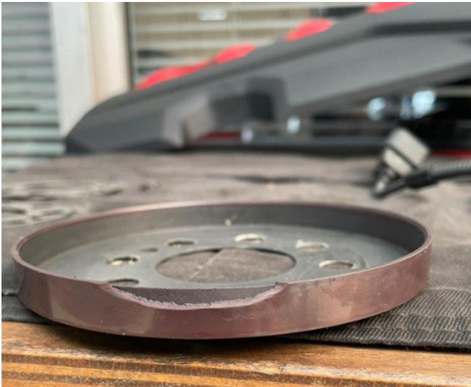
Figure 2. Damaged sensor wheel uninstalled.
