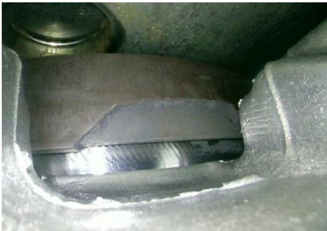
Figure 1. Damaged sensor wheel in installed position.
