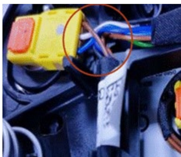
Figure 2. Tension on connector for airbag release valve igniter.
