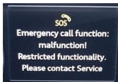
Figure 1. Emergency call malfunction warning.
