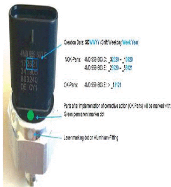
Figure 1. Pressure and temperature sensor markings and build date.
