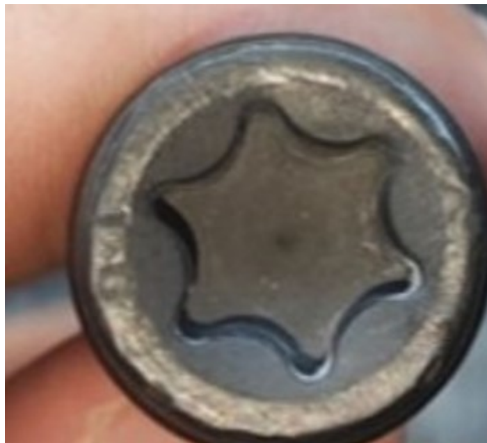
Fig. 2 Incorrect Head Fastener
