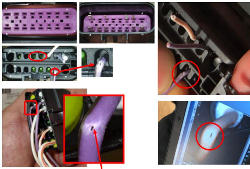
16-Way XY101A Inline Connector Damage
