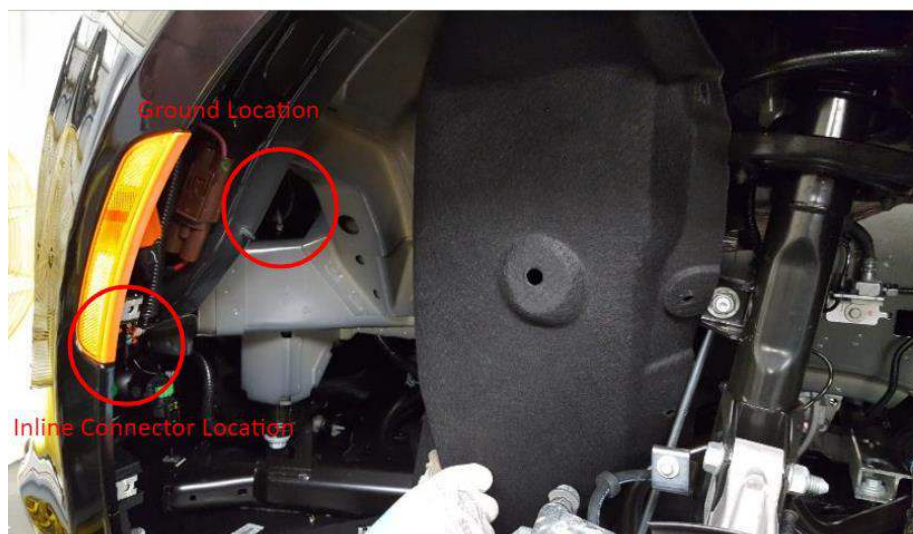
Ground and Inline Locations
