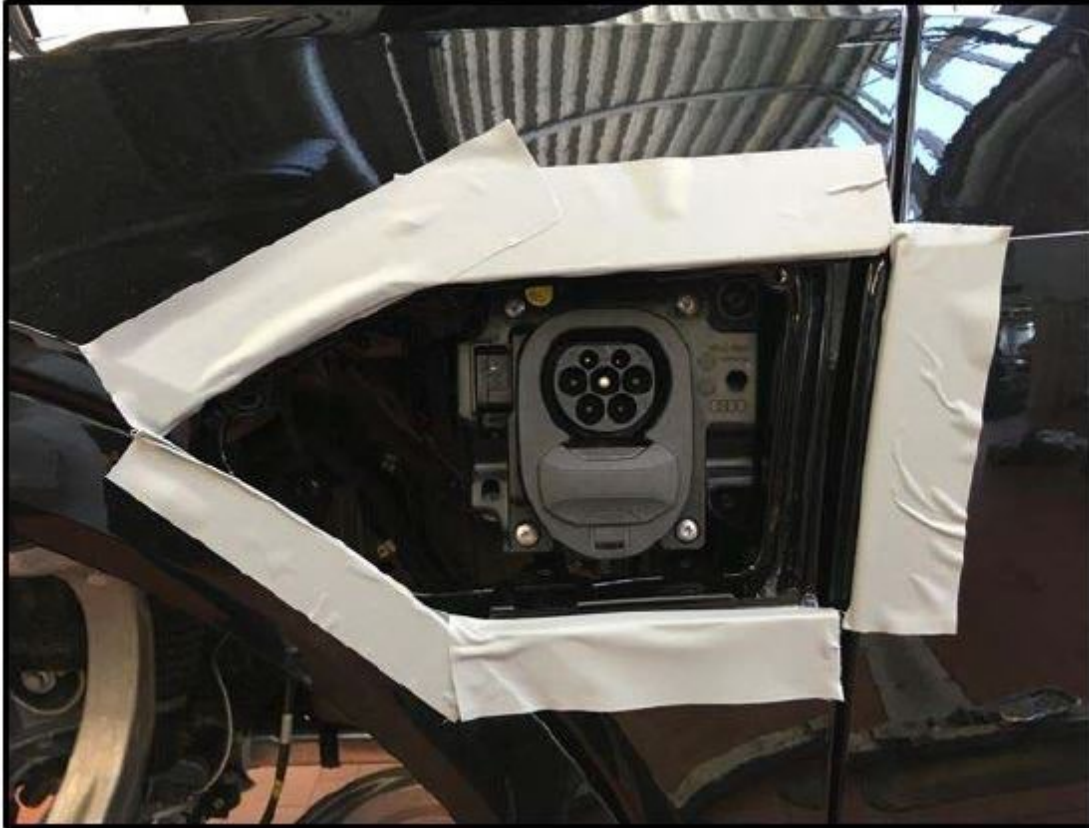
Figure 18: Adhesive tape applied around the charging door to protect the paint.
