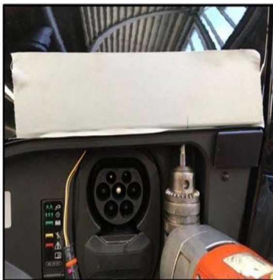
Figure 12: Use an angled drill/angle bit to drill to a depth of 15mm at the marked location.
