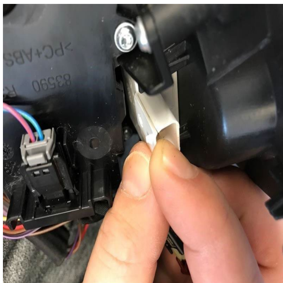
Figure 1: Crack in the connector point of the charging indicator.
