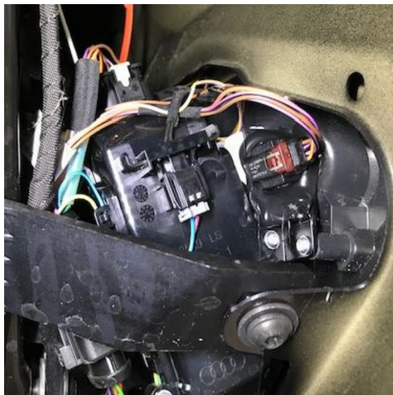
Figure 24: The connector should be completely surrounded by the adhesive sealant.
