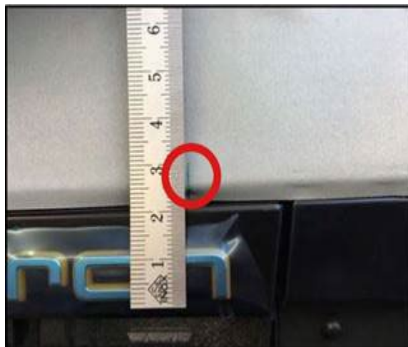
Figure 10: Make a vertical mark in the middle of the “n” of the e-tron emblem.
