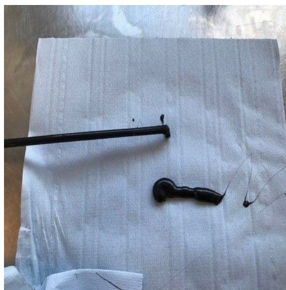
Figure 22: Clearing the component adhesive sealant after prolonged storage.
