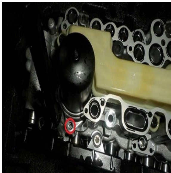
Figure 5. The bolt head is missing.
