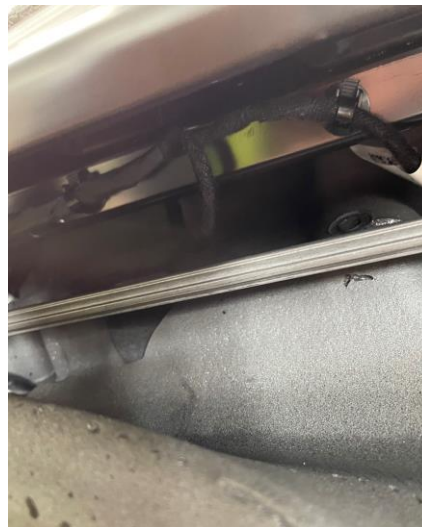
Example of proper routing in 2 nd row Seatback
