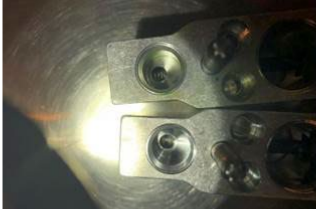
Figure 4. Leak at expansion valve connection evidenced by residue from the contrast agent.
