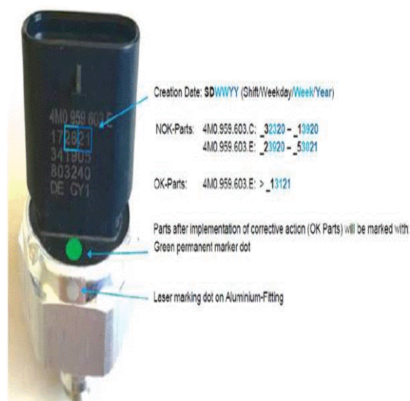
Figure 1. Pressure and temperature sensor markings and build date.
