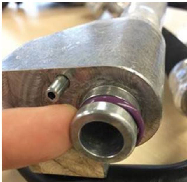
Figure 1. Damaged refrigerant line O-ring seal.
