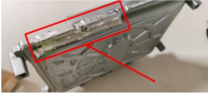
Fig. 2 Foil Tape At PCM
