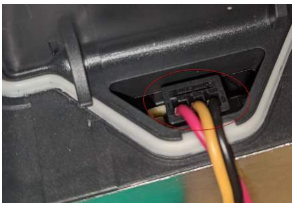
Figure 3. Backup battery connector (no release mechanism).
