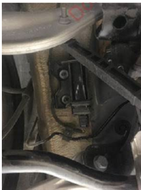
Figure 1. Installation location with standard bracket 4K0 907 249 A.
