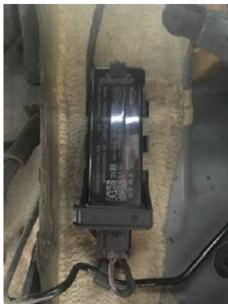
Figure 2. Installation location with new bracket 4E0 810 675 B.
