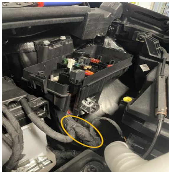
Figure 1: J1 splice point location.
