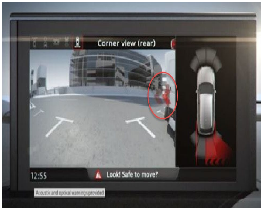
Figure 1: RCTA/Intersection assist arrows.
