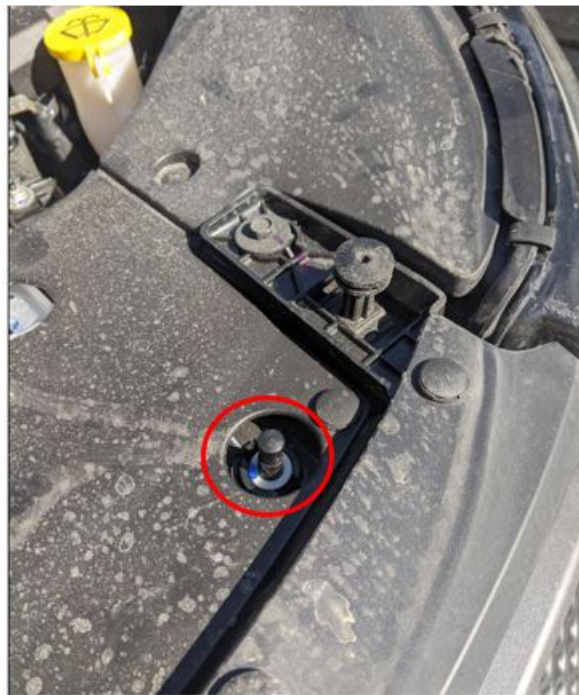
Fig. 1 Hood Switch Location
