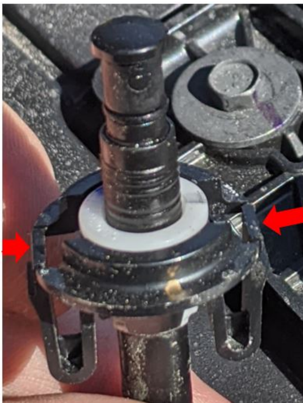
Fig. 1 Plunger Style Switch
