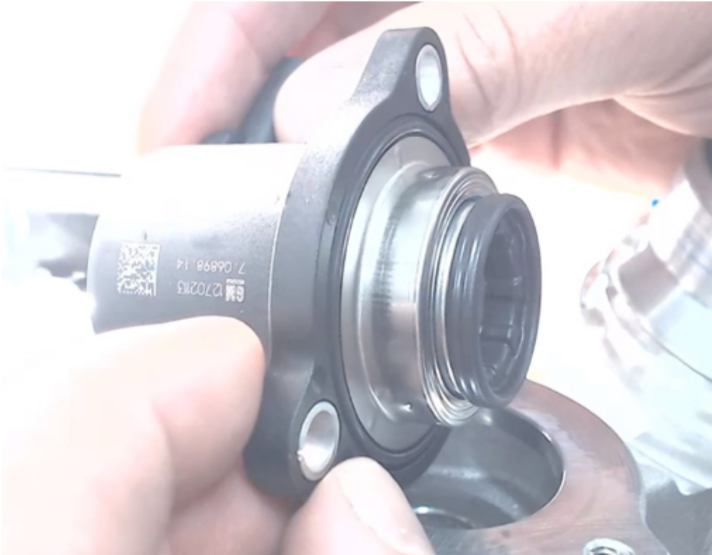
Picture below shows Charge Air Bypass valve fully extended or closed position
