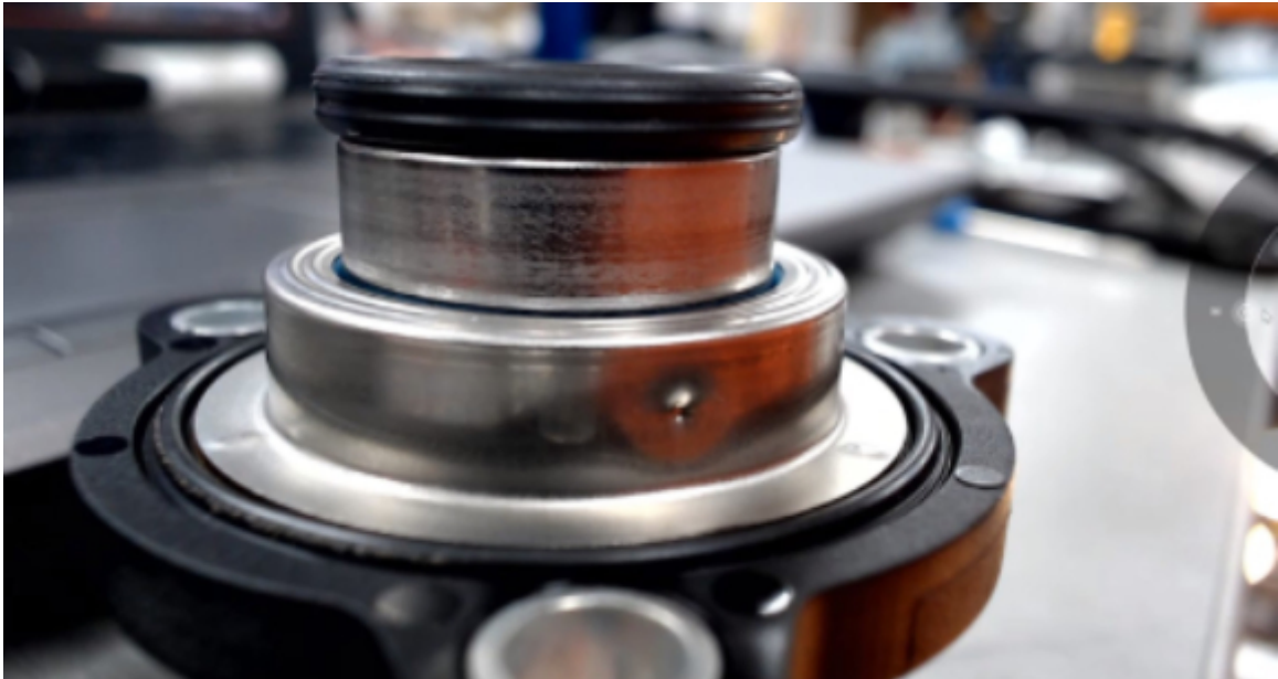
Picture below shows Charge Air Bypass valve fully extended or closed position
