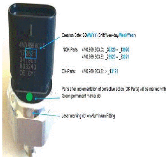
Figure 1. Pressure and temperature sensor markings and build date.
