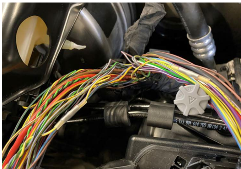
Figure 2: Wires isolated for modification.
