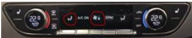
Figure 7. 72° f (22° c), Sync, air distribution to footwell, medium blower speed.
