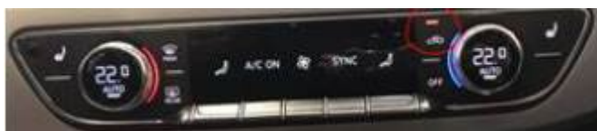
Figure 5. Auto, 72° f (22° c), Sync, air recirculation mode.
