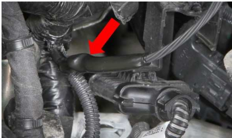
Fig. 3 Shrink Wrapped Wires
