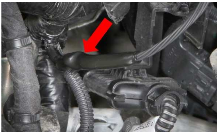
Fig. 3 Shrink Wrapped Wires
