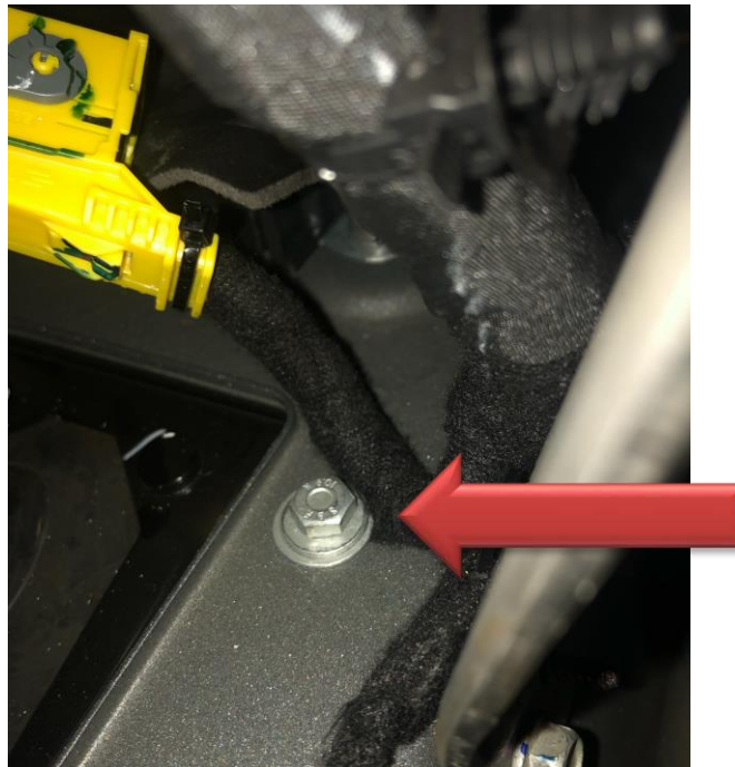
Wiring Harness Crushed Under Bolt
