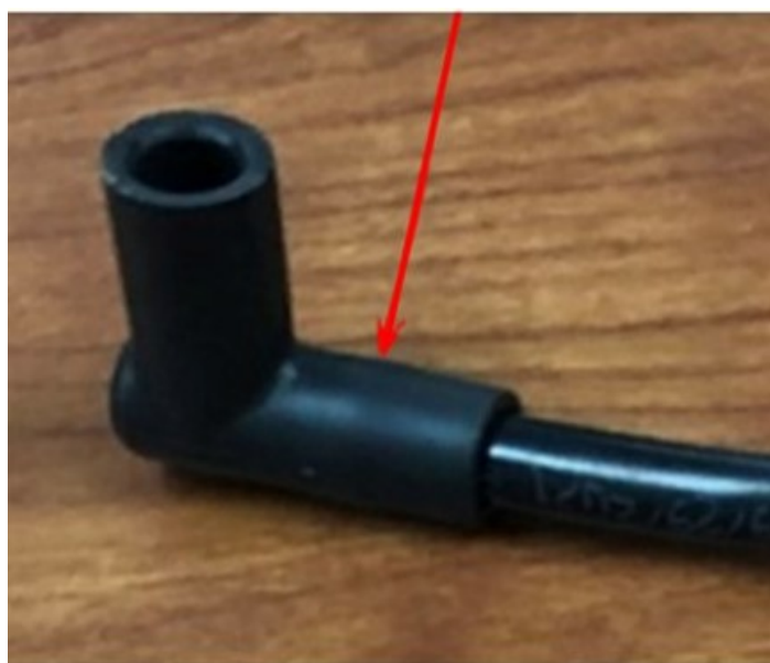
Fig. 2 Purge Tube Inserted Too Far
