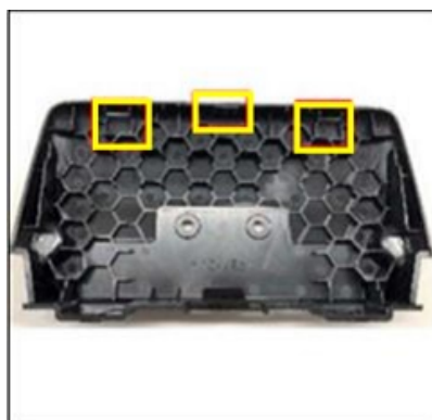
Rear cover (joint with center display)
