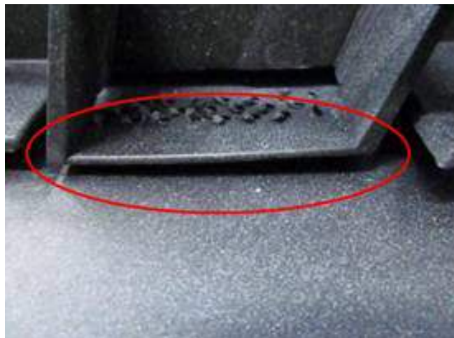
Figure 4. Loose mounting bracket.
