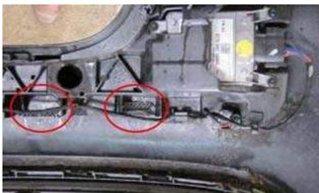
Figure 2. Mounting bracket for one of the ECUs.
