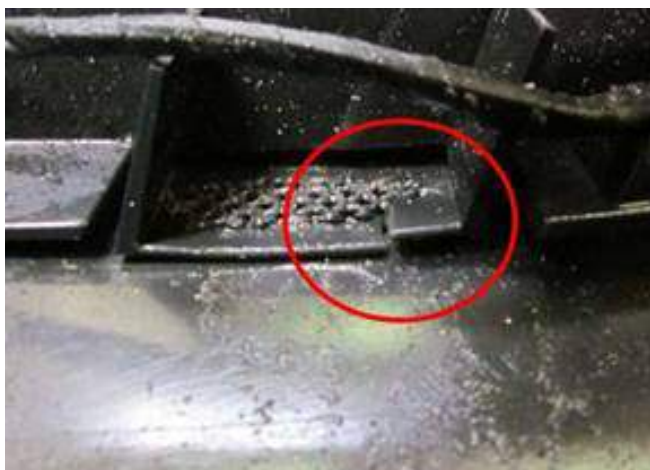
Figure 3. Broken mounting bracket
