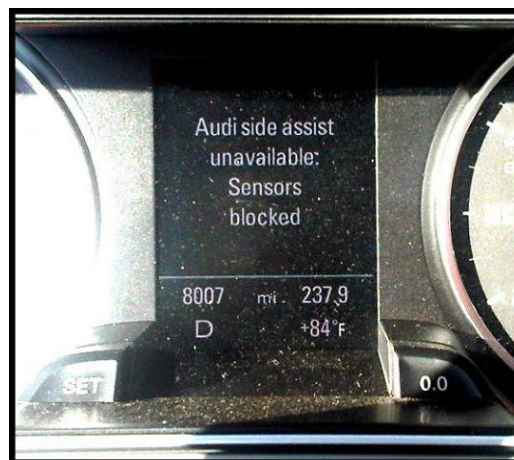
Figure 1. Audi Side Assist warning in DIS
