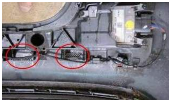
Figure 2. Mounting bracket for one of the ECUs.
