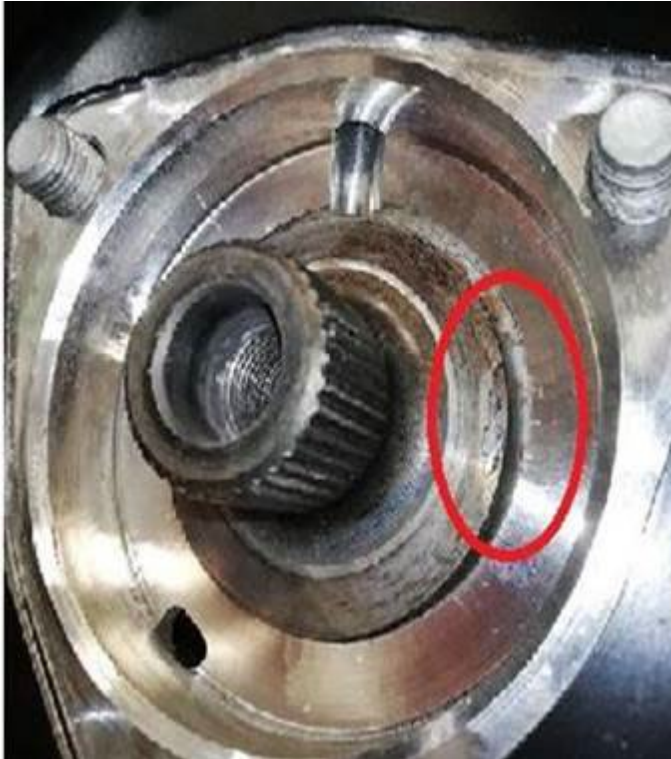
Figure 4: Metallic particles/damage in the wheel hub/bearing.
