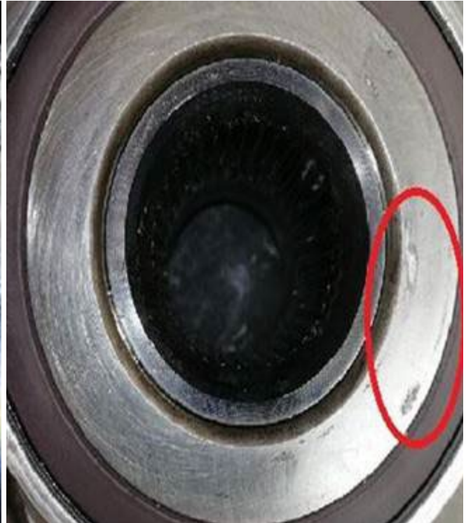
Figure 5: Metallic particles/damage in the wheel hub/bearing.
