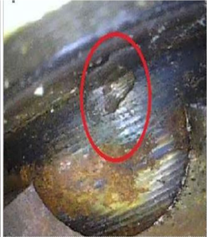
Figure 3: Metallic particles in the hub.
