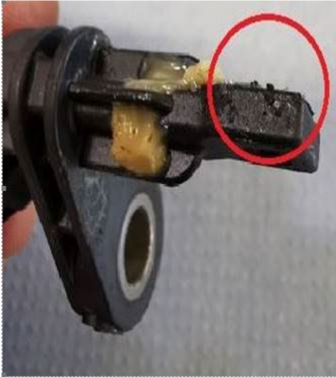
Figure 2: Metallic particles in the speed sensor.
