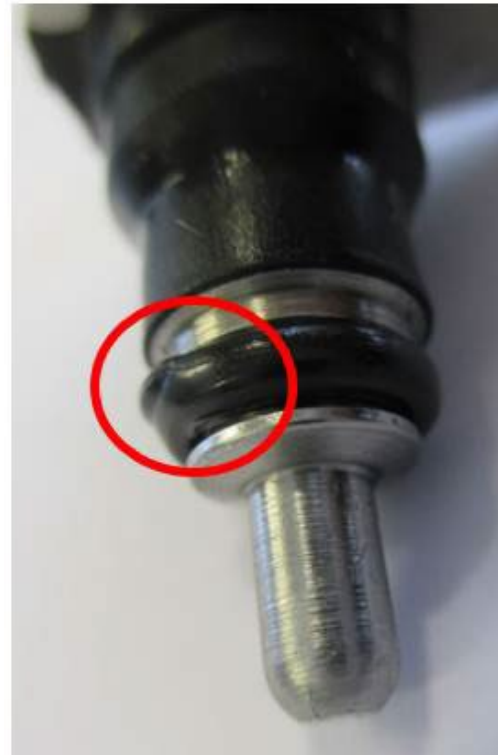
Figure 1. O-ring is pinched.
