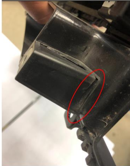
Fig 1 Broken ACC mounting pedestal.
