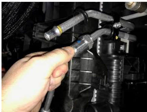
Fig. 3 Transmission Oil Cooler Line (Connected)
