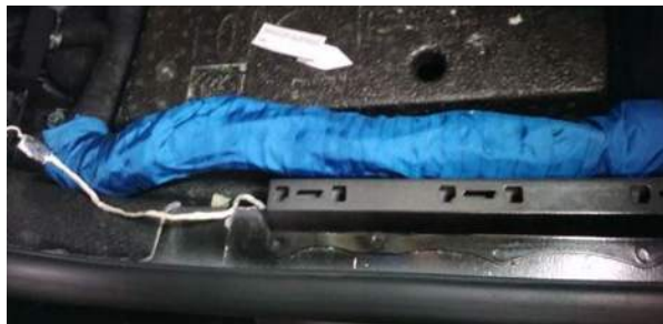
Figure 10: Main wiring harness wrapped with blue textile tape.
