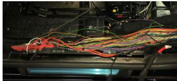
Figure 2: Driver side door sill area, open harness to expose splice points.
