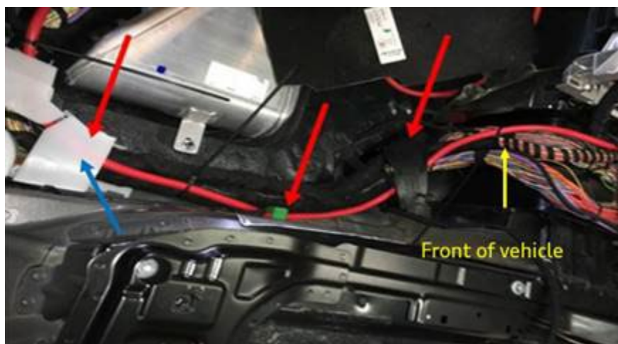
Figure 8: Routing path passenger side. The lower portion of the photo is where the sea bottom mounts.
