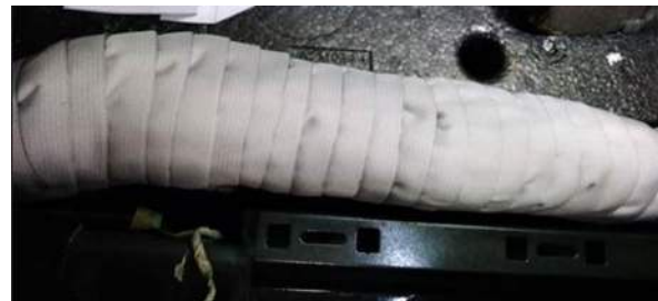
Figure 11: Gray textile tape covering the already wrapped main wiring harness.
