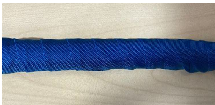
Figure 6: Cable wrapping for N 107 292 04 (blue).
