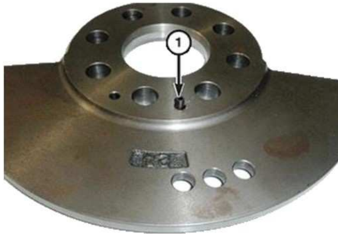
Fig. 3 Counter Weight Dowel Pin Location
