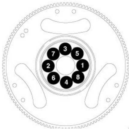
Fig. 4 Flex Plate Bolt Sequence
