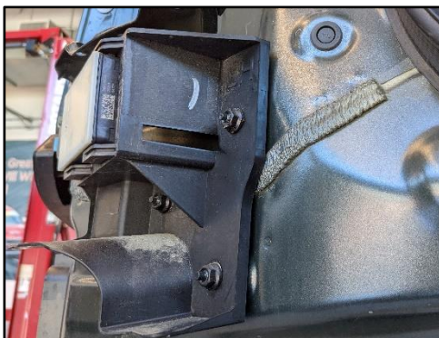
Rear corner radar unit bracket body sealer interference.
