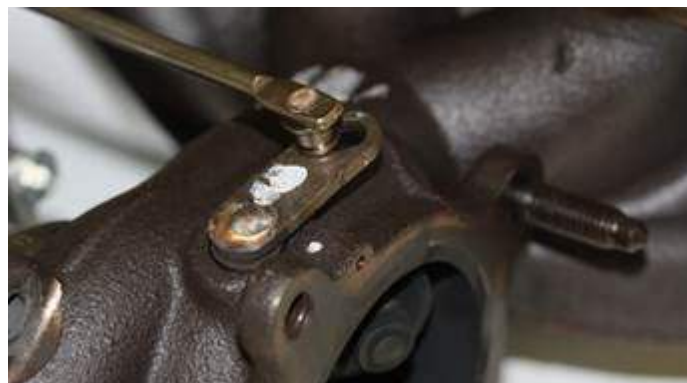
Figure 1. Disconnected wastegate linkage.
