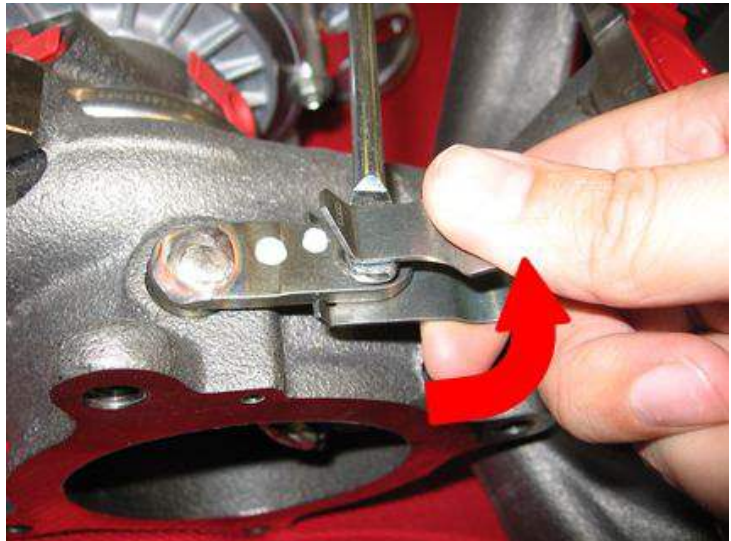
Figure 2. Turn the clip counter clockwise till the lugs slot in.
