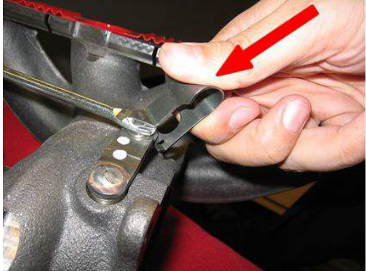
Figure 1. Fit the clip from the side.
