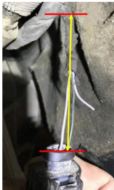
Figure 2. Measure 110 mm from T3r to the first harness branch
